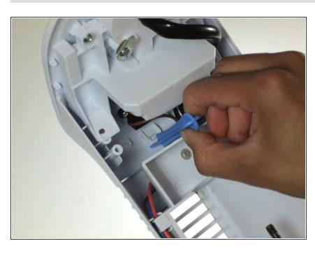
Pry off the control panel by forcefully lifting the tab located inside the front of the fan with the plastic opening tool. To reassemble your device, follow these instructions in reverse order.
