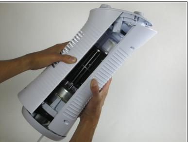
Pull the front and back parts of the case away from each other until the back is free from the front.
