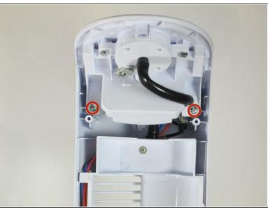
Remove the two 3mm screws found just below the top of the device using the Phillips #0 Screwdriver.
