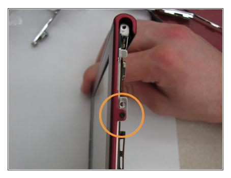
Using the same screwdriver, remove the 1.4 mm screw at the bottom of the device that is usually covered by the bottom and side panel.
