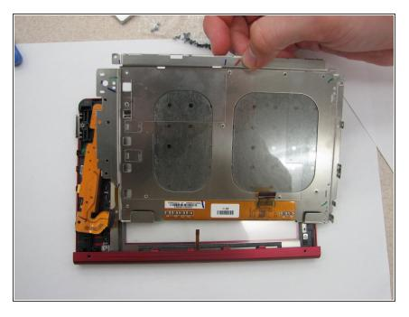
• Lift the end of screen opposite the red edge and pull it out of the casing.
