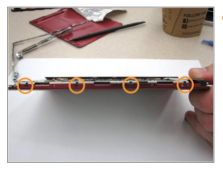
Remove the four 1.4 mm screws that are located on the side of the device that are usually covered by the bottom and side panel.
