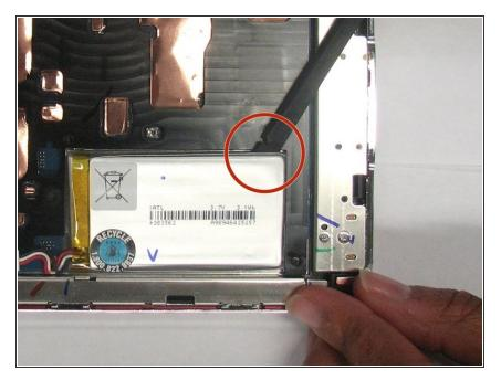
Use the flat end of the spudger to pry the battery out of its holder.
