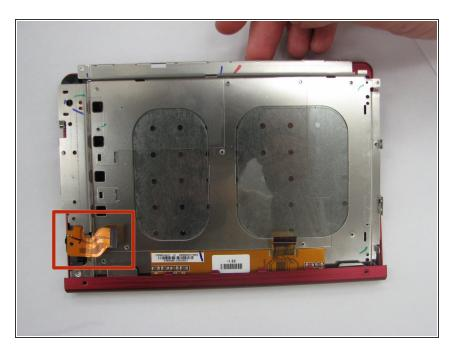
Be sure to lift the thin, orange strip that is attached to the audio/AC/mini USB ports out of the way, before removing the screen.
