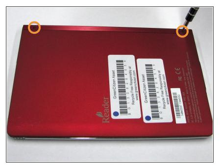
Using the Phillips head screwdriver PH000, remove the two 1.4 mm screws that are located on the backside of the device.
