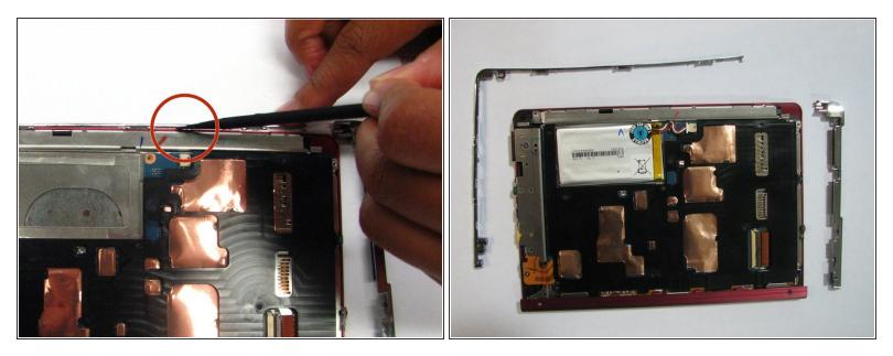
• Pull the panel away from the device. You may have to use the flat end of the spudger to remove the side portion of the panel because it will be glued in place.
