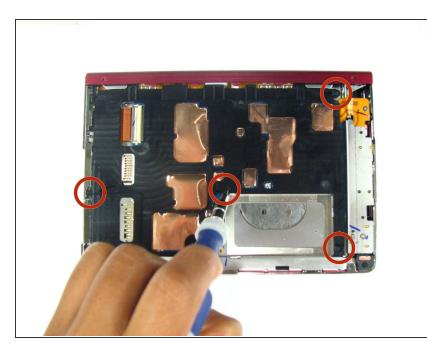
Using a screwdriver remove the four
