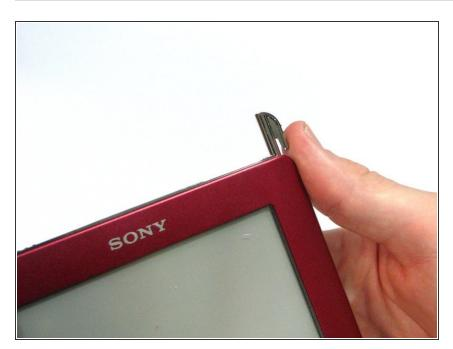
• Remove the stylus from the device.
