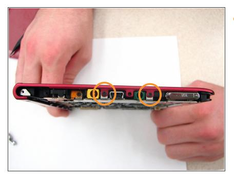
Using the Phillips head screwdriver, remove the two 1.4 mm screws in the screen at the bottom of the device that are usually covered by the power switch panel.
