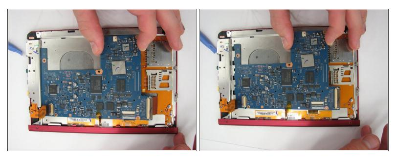
• Lift the end of the motherboard closest to the memory cards and pull out.
