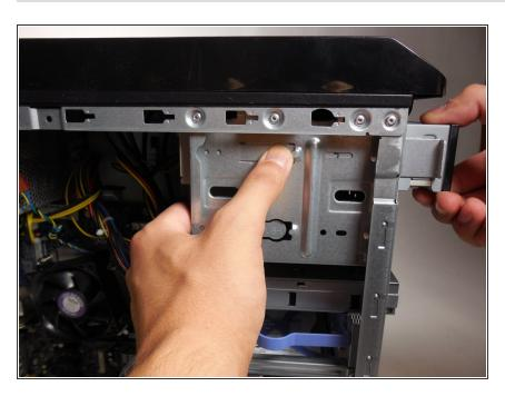
Push down on the button that says "push" while pulling the optical drive outward. To reassemble your device, follow these instructions in reverse order.
