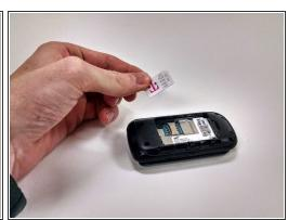
Using your thumb, slide SIM card out toward the base of the phone
