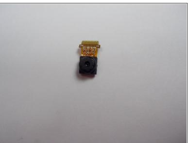
• Use tweezers to pick up the ribbon wire, and lift. The frontward facing camera will follow suit.
