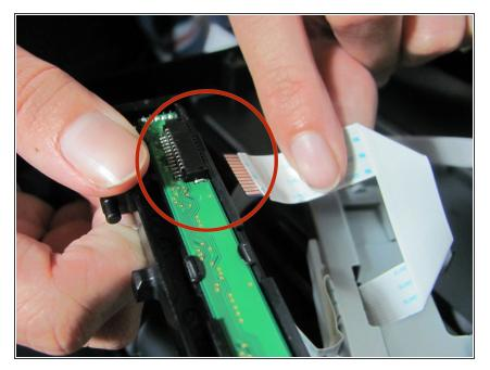
Now that the scanner light assembly is free. Lift it out of the scanner bed and unplug the large white wire that attaches it to the rest of the printer.
