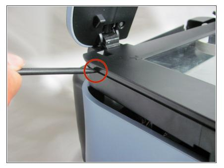
• You will have to pry off the glass cover lid. There are no screws that you have to worry about. Just insert a spudger into the crack between the glass lid and black base as shown.
