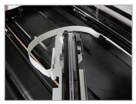
After lifting the glass cover up, the light assembly will come free because it was only held in place by the glass top.
