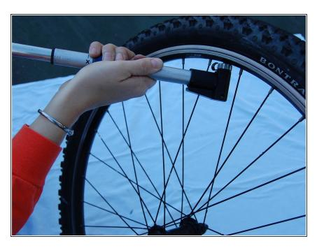
To deflate the tire, remove the cap and attach the pump head to the valve. You should then hear air flowing out from the tire.
