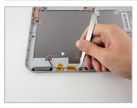
Using either your hands or tweezers remove the 3 pieces of tape holding the speaker wires to the back panel.
