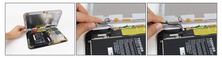
• Remove the speaker cable from its socket by gripping both sides of the white connector piece with <u>tweezers</u> and pulling straight out.
