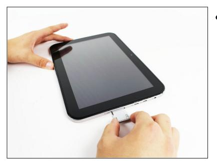
• Remove the SD card from the SD card slot.
