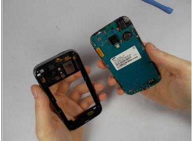
• Use the pry tool to pry the back panel from the rest of the phone. Pry from the edge closest to the screen for simplicity.
