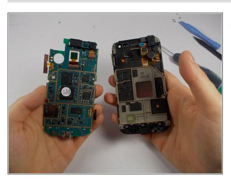
Lift the motherboard upwards separating it from your screen.
