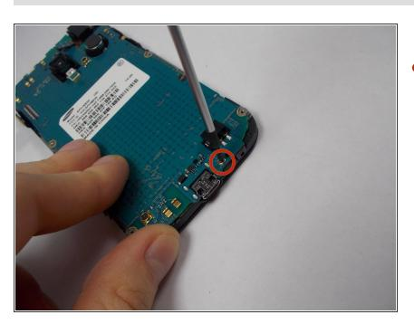
Use a philips-head screwdriver to remove the single screw on the bottom of the phone. Located to the right of the charging port.
