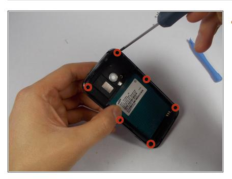
With a small phillips-head screw driver, remove the six screws holding the back panel in place.
