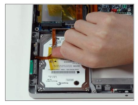
Peel up the orange ribbon cable taped to the top of the hard drive. This cable is still connected to the hard drive, so you will only be able to lift up on the cable a little.
