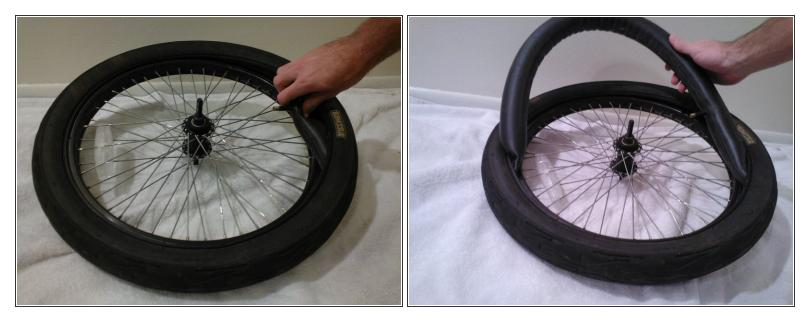
Beginning with the nozzle, remove the damaged inner tube by pulling it out from in between the tire
