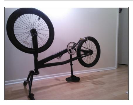
Flip the bike over so that only the handle bars and the seat are touching the ground
