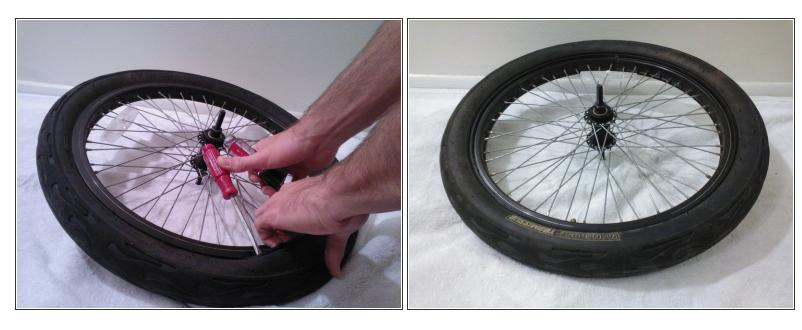
Place your fingers in between where the tire is already overlapping the rim and pry out the rest of the tire so that the whole tire overlaps the rim.
