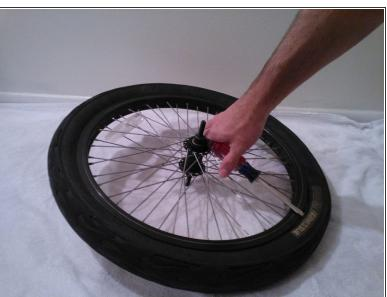
• Wedge a screwdriver between the tire and the rim to pry it over the tire over the rim as shown. Part of the tire should now be on top of the rim.
