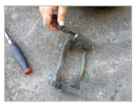
Pull the boot from the caliper bracket and slide the pin out to inspect. If there is heavy pitting or rust, you will want to replace the slide pins and bracket. Otherwise, lube with brake lubricant grease for reassembly.
