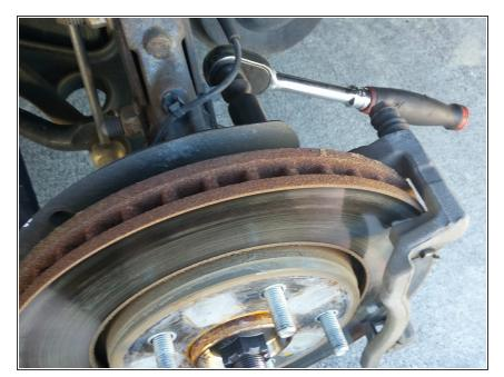
Using the ratchet and socket (21mm for the front, 18mm for the rear), and remove the bolts holding the caliper mounting bracket. Again, it may be helpful to loosen both bolts before complete removal.
