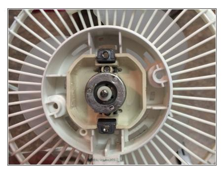
Now that the old motor is removed, a new motor can be placed in the motor housing.
