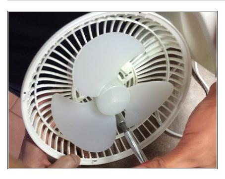
Remove the 3 screws holding the fan on to the motor housing using a 3/16" philips head screw driver. The
