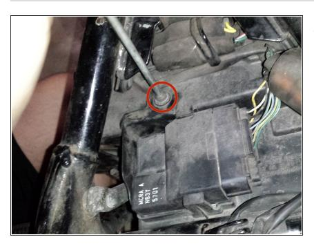
Using the screwdriver, remove the screw holding the plastic cover.
