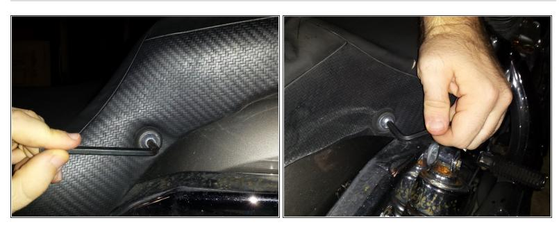
Using the allen wrench, remove the screws on both sides of the bike seat.
