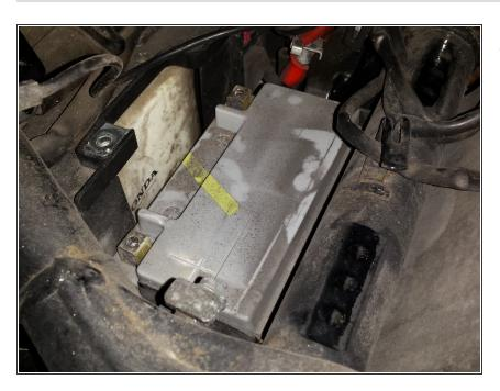
Remove the battery from the bike by pulling upwards.
