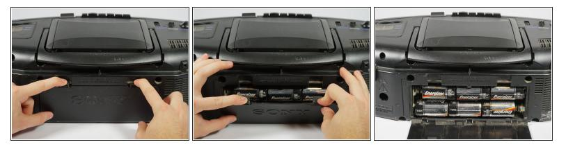
Remove the battery cover on the back of the boombox by applying downward pressure to the two clamps.
