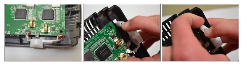
• Apply pressure with your finger to the black tab that retains the refresh button while using your other hand to pull the bottom of the refresh button from the post.
