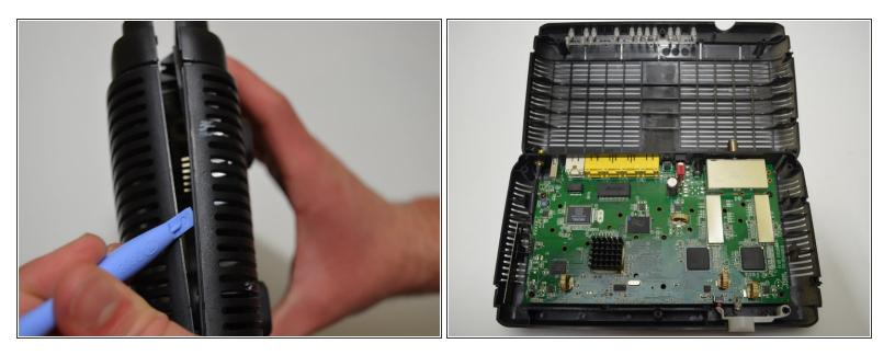
• Use a plastic-opening tool and pry the top casing from the bottom casing to expose the circuit board in the bottom half of the device.
