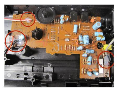
Remove the epoxy completely from the motherboard so that the wires underneath the epoxy can move freely.
