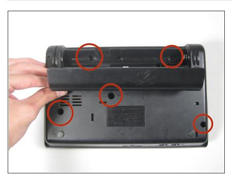
Remove the 5 5.95mm screws as indicated in the picture using the Phillips Head screwdriver.
