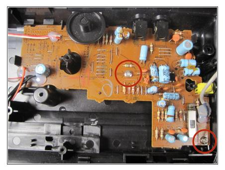
Remove the 2 5.95mm screws as indicated by the picture using the Phillips Head screwdriver.
