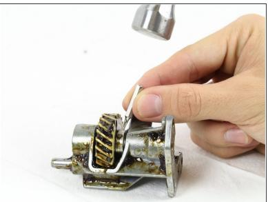
Using a pin punch and a hammer, remove the roll pin.
