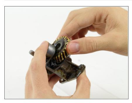
Remove the worm gear from the tower.
