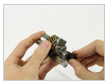
Slide the tower gear out to access the worm gear.
