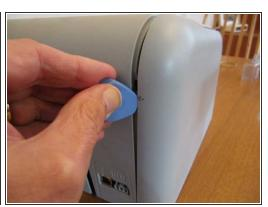
Prise off the left hand side panel. First, release 2 clips at the top and one at the back.
