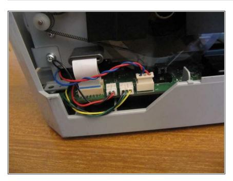
From the left hand side near the rear of the printer, disconnect 2 ribbons, one behind the other, and 3 wire connectors.
