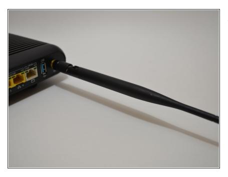
Lower the antenna so that it is parallel to the table surface.
