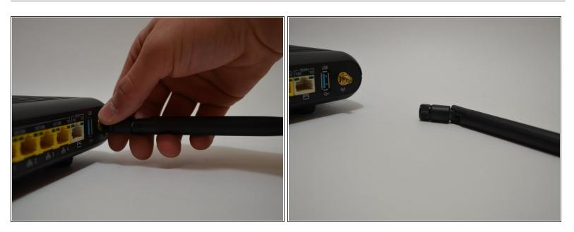
Unscrew the antenna counterclockwise at the threaded base until it is detached.
