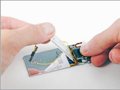
Use your fingers to carefully lift the battery off the back of the LCD, starting at the top of the LCD.
