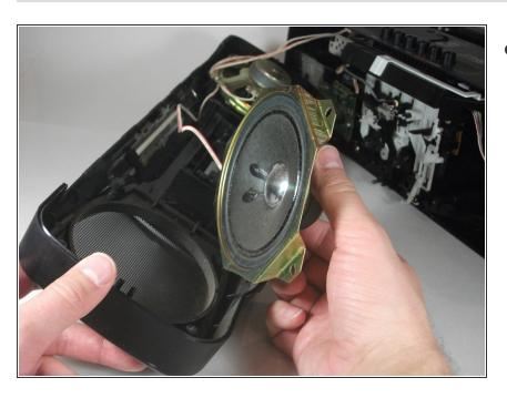
Lift the speakers out of the front face of the radio to complete the removal.
