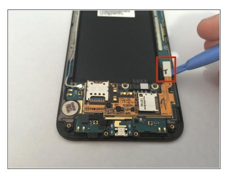
Using your plastic opening tool, disconnect the connection between the phone and the ribbon cable.
