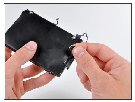
Remove the strip of tape covering the hard drive connector.
