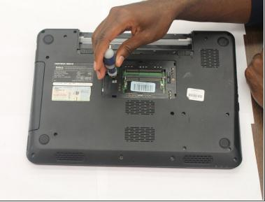
Remove the 6 mm Phillips #000 screw using the Phillips #000 Screwdriver.
