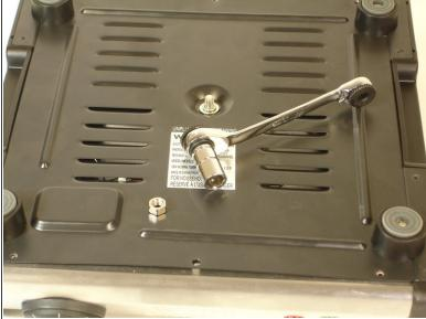
Using a wrench, remove the bolt from the center of the back panel.
