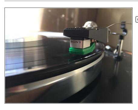
Once the needle clicks into place, test the record player to ensure that the needle works properly.
