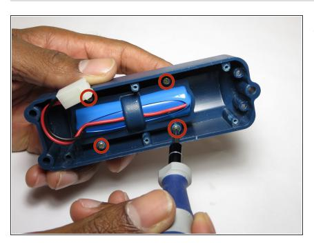
Remove the four #0 15mm screws to release the battery housing from the case.
