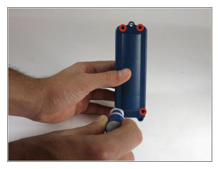
To open up the casing, you will need to unscrew the four Phillips #0
