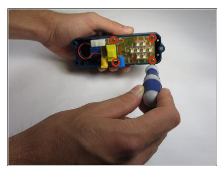
Unscrew the Phillips four #0 15mm screws to free the motherboard from the casing.
