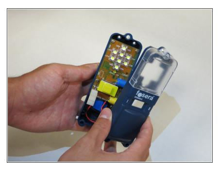
Gently separate the two halves of the casing.
