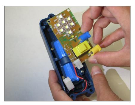
Slowly pull the motherboard out of the casing. Make sure the loose battery wire doesn't get snagged.
