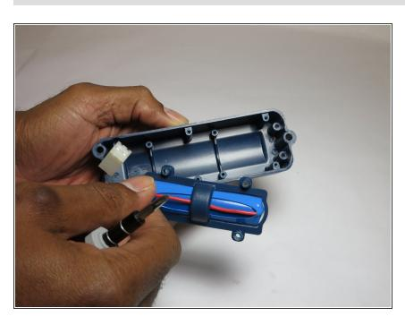
Take the battery housing and battery out of the casing.
