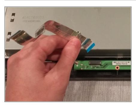
Remove the Flat Flex Cables from the Power Button Circuit Board.
