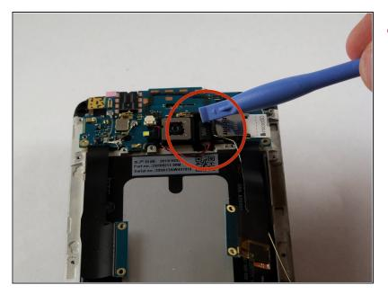
Pick up and set aside vibrator, do not disconnect.
