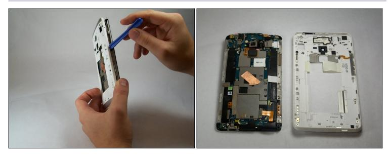
• Use the small plastic opening tool to pry between the screen and the rear case.
