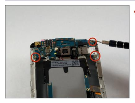
• Remove the three 3 mm Phillips #000 screws from the secondary board at the top.
