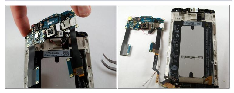
• Lift the secondary motherboard with the camera attached.
