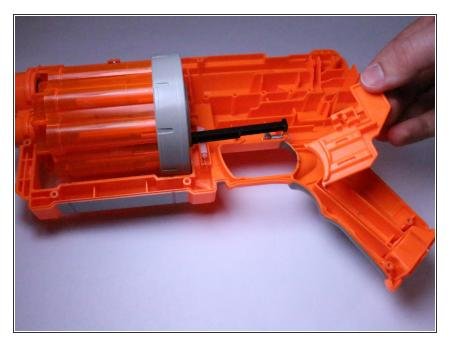
Once the black piece has been detached, the trigger can be lifted out of the device.
