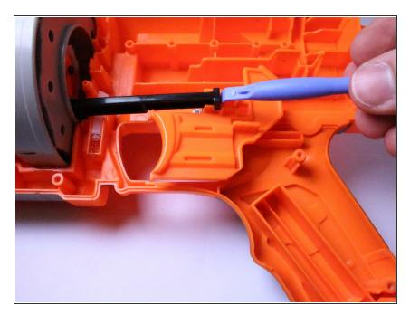
Using a plastic opening tool, detach the black piece from the trigger. You do not need to remove the black piece from the gun.
