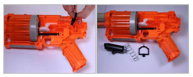
Using your hand, lift the large spring and attached plastic stabilizing piece out of the gun and set aside.
