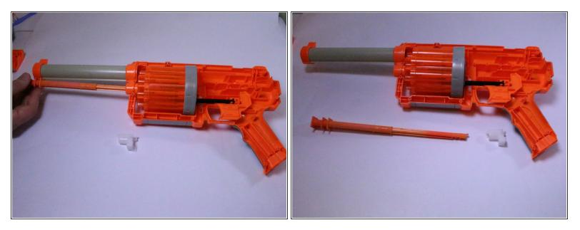
• Using your hand, slide the track out of the gun by pulling it away form the device.
