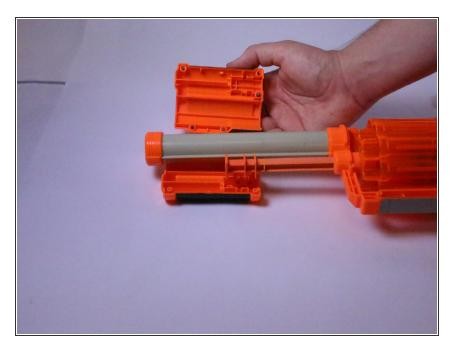
Once all of the screws have been removed lift the pump handle off and set it aside.
