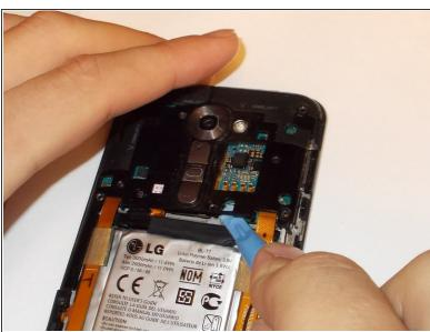
After all visible screws have been removed use the spudger to pop off the top plastic cover.
