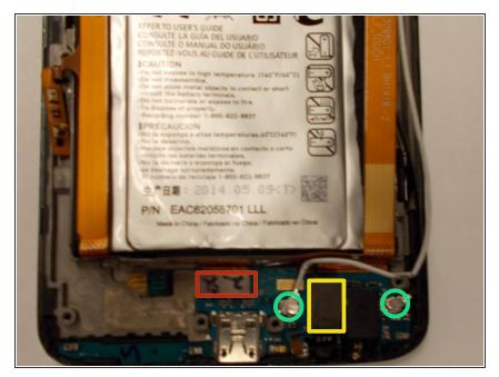
Disconnect the 2 connectors. The LCD connector (red color coded) and the Digitizer (yellow color coded). Together with these 2, remove the 2 antenna connections (green color coded) also.
