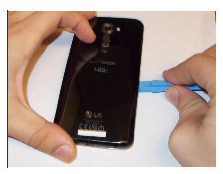
Using the plastic opening tool, or the thin side of the spudger to separate the back cover from the phone. Start at the bottom corner of the phone.
