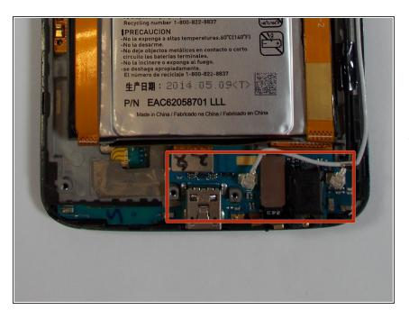
It may seem as if the flex cable are free to remove, but not yet. The two flex cable are both together at the bottom, and connected to a small control board. Therefore we need to remove the control board completely.
