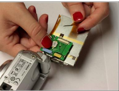
Locate the ribbon (orange) and using tweezers gently pull back the retaining clip and pull the ribbon out
