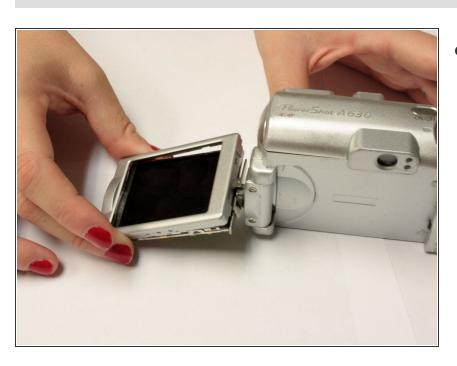
Gently remove front panel of the LCD screen
