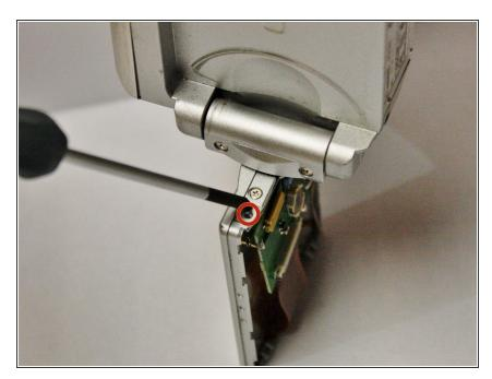
Once the back panel is removed another .2mm screw will be revealed, remove this screw to remove the front panel of the LCD screen
