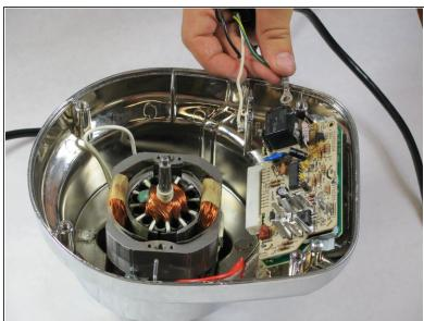
Using the Phillips #2 screwdriver, remove the #8 Phillips 6mm screw to which the green wire is attached.
