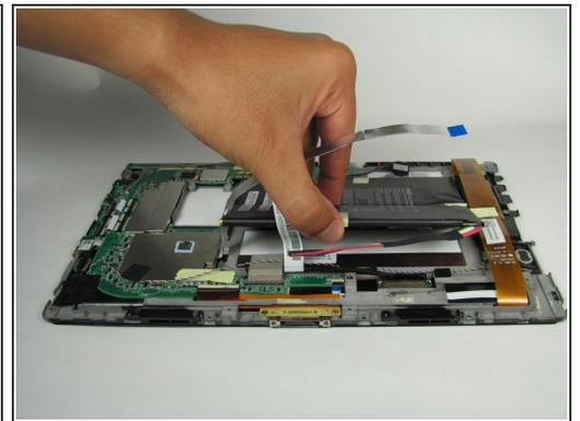
**i** Battery is glued to device. Remove with care.
