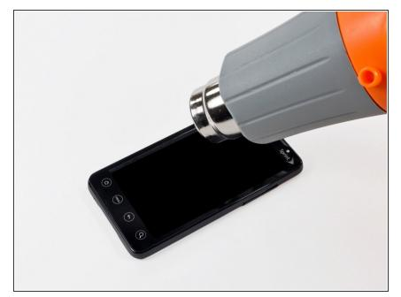
Use a heat gun to soften the adhesive along the left side of the front glass panel.
