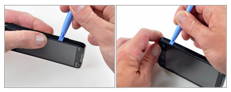
Insert the iPod opening tool between the front panel and its plastic surround and pry up at several points along the left edge of the Evo.
