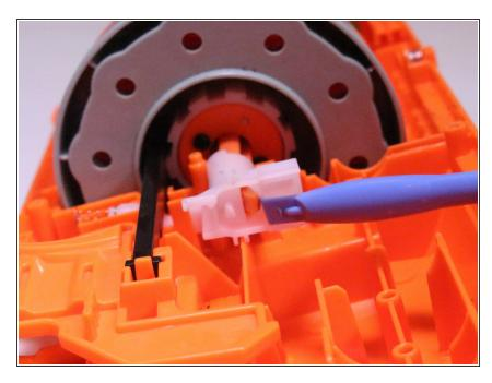
Using a plastic opening tool, lift the white piece out of the gun and set it aside.
