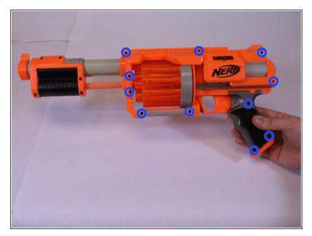
Using a 00 Phillips screwdriver, remove all screws from the front panel. The screws have a length of .95 cm.
