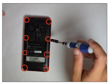
• Remove eight 8.3mm T4 screws with the Torx screwdriver.
