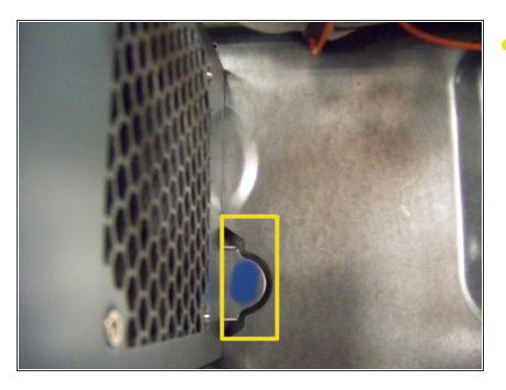
Press the blue release button. This is located on the floor of the computer chassis right in front of the power supply.
