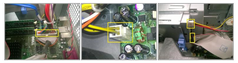
• Gently disconnect the power cables from the motherboard and drives.
