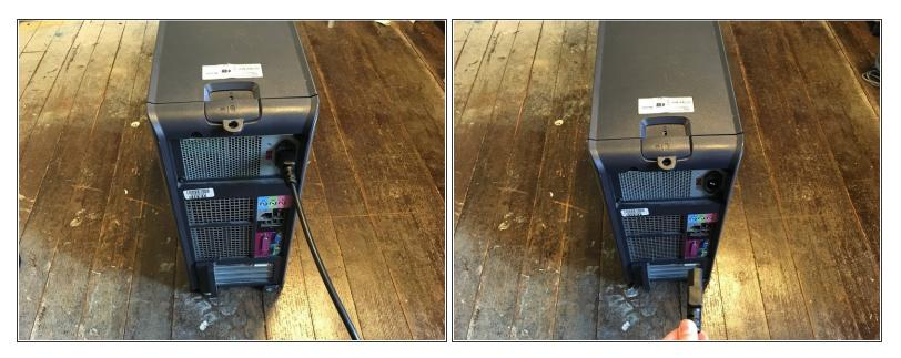
• Power down your PC and remove the power cord from the back.
