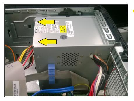
Remove the unconnected power supply by sliding it towards the front of the computer. Next, lift it up out of the chassis.
