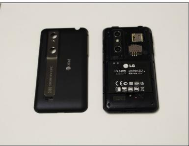
Pry the back cover off of the phone with your fingernail. There is a notch located at the bottom of the phone for improved leverage.
