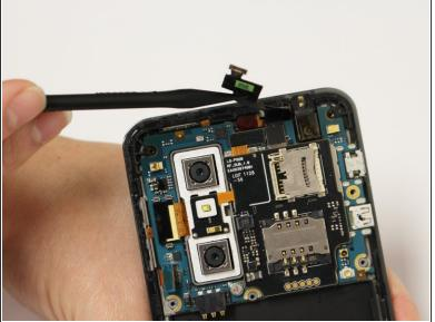
Using a spudger or plastic opening tool, gently disconnect the ribbon cable attached to the black SIM card board.
