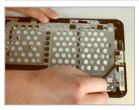
With a spudger, disconnect the cable connecting the camera to the motherboard.
