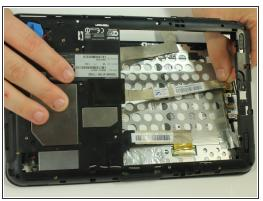
Once the back of the case is off, disconnect the wires by gently pulling on the plastic tabs as shown.
