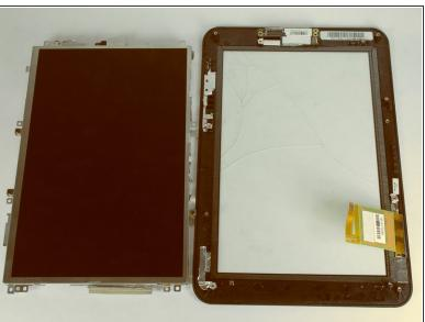
Lift up the LCD from the screen and place it on the side
