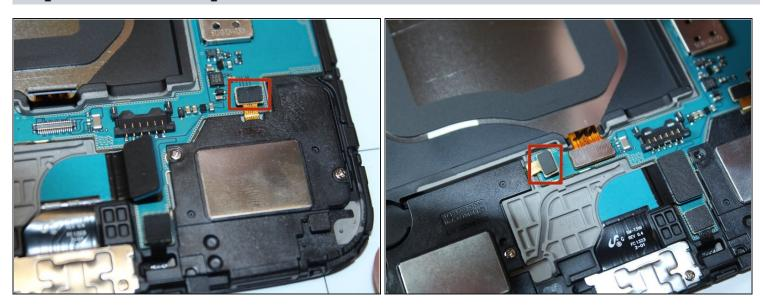
• Disconnect the relays attached to the motherboard.
