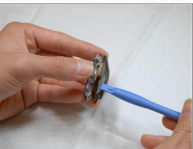
Open the case by inserting the plastic opening tool into the seam of the device.
