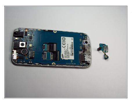
Once its released, gently lift the main board and remove the USB board containing the charging port.
