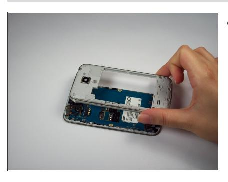
Carefully separate the rear housing and the mid-frame to reveal the inside of the phone.
