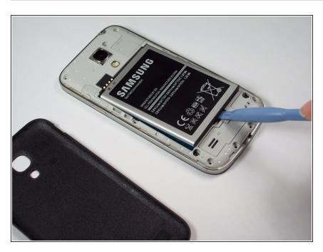
Pry the battery out using a plastic opening tool.
