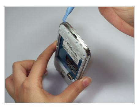
Starting at the USB port, slide a plastic tool around the perimeter of the phone between the rear housing and frame. As you work your way around the edge you will feel the clips release.
