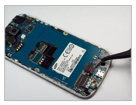
Remove the 2 flex cables shown that attach to the USB board, Tweezers can be especially helpful here.
