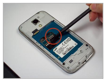
Using a nylon spudger, push through the hole at the top of the memory card holder to slide it out.
