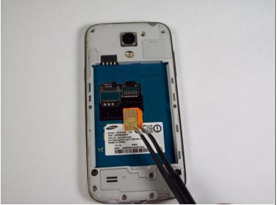
• Using tweezers, remove the SIM card by sliding it towards the bottom of the device.
