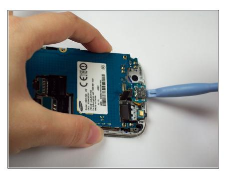
Gently pry underneath the charging port using the plastic opening tool to separate it from the double sided tape below.
