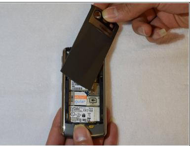
Turn the phone over so that the screen is facing the table. Locate the chrome release button and push it in to unclip the battery cover.
