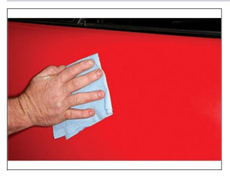
Finish with light hand buffing to remove the last of the compound. Follow with car wax.
