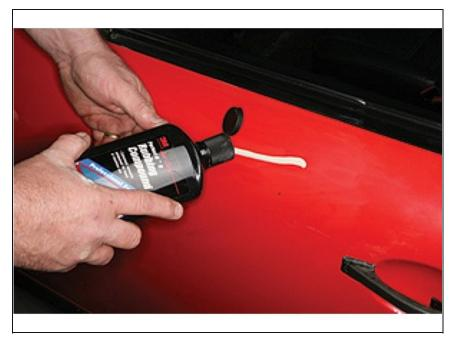
Polish out the sanding scratches with rubbing compound.
