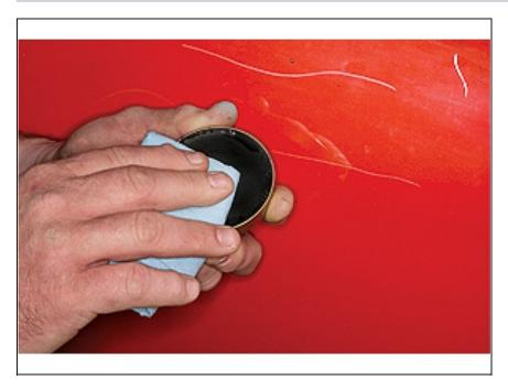
Shoe polish can be used to visualize the scratches. Rub a small amount of dark shoe polish over the scratch.
