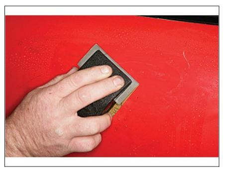
Block sand the panel with 2000-grit wet/dry sandpaper and plenty of water. Sand until the shoe polish disappears.
