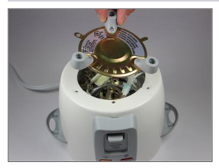
• Lift the brass plate off the device and set it aside.
