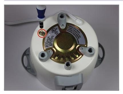
Using a spanner screwdriver, remove the one 10mm long 7mm diameter spanner screw from the side of the brass panel.
