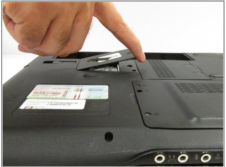
**!** Make sure your computer is powered down and unplugged from the charger before removing any components.
