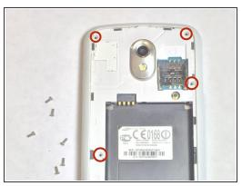
Remove 4.4 mm screws using a PH # 000 as indicated on the picture.
