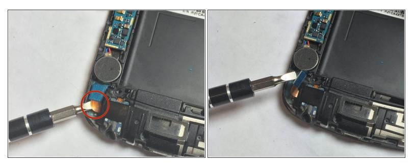
With the flat head screw driver pull up the blue connector.
