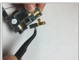
Using tweezers pull the top earpiece out.
